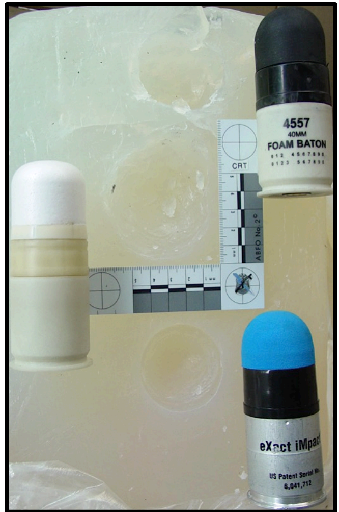
From Top: CTS 4557 , SDI's BIP and eXact iImpact fired into MBM at 10 feet
