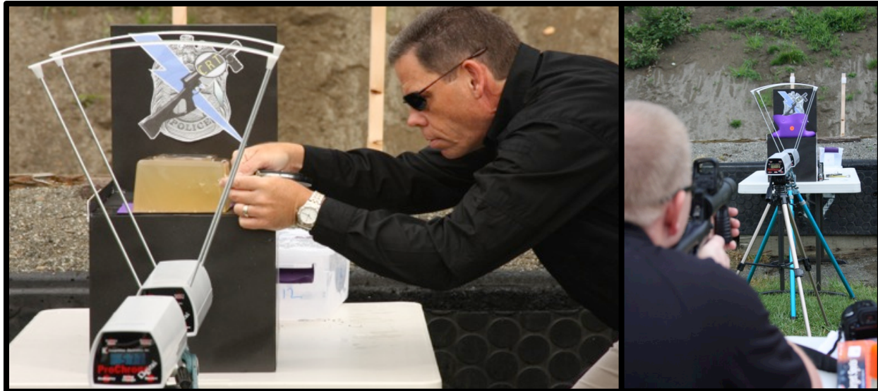
BIP Fired into Covered (3 mm Neoprene) 10% Ballistic Gelatin
